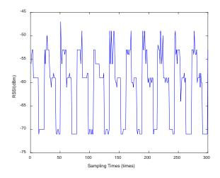
Figure 1. Fluctuation diagram of RSSI signal received at a distance of 1m
