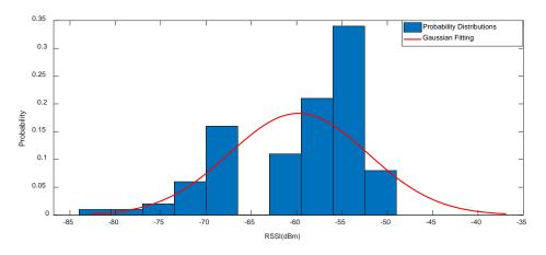
Figure 2. Gaussian distribution of RSSI value at 1m
